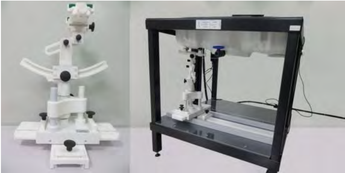
Device holder supplied by SATIMO
