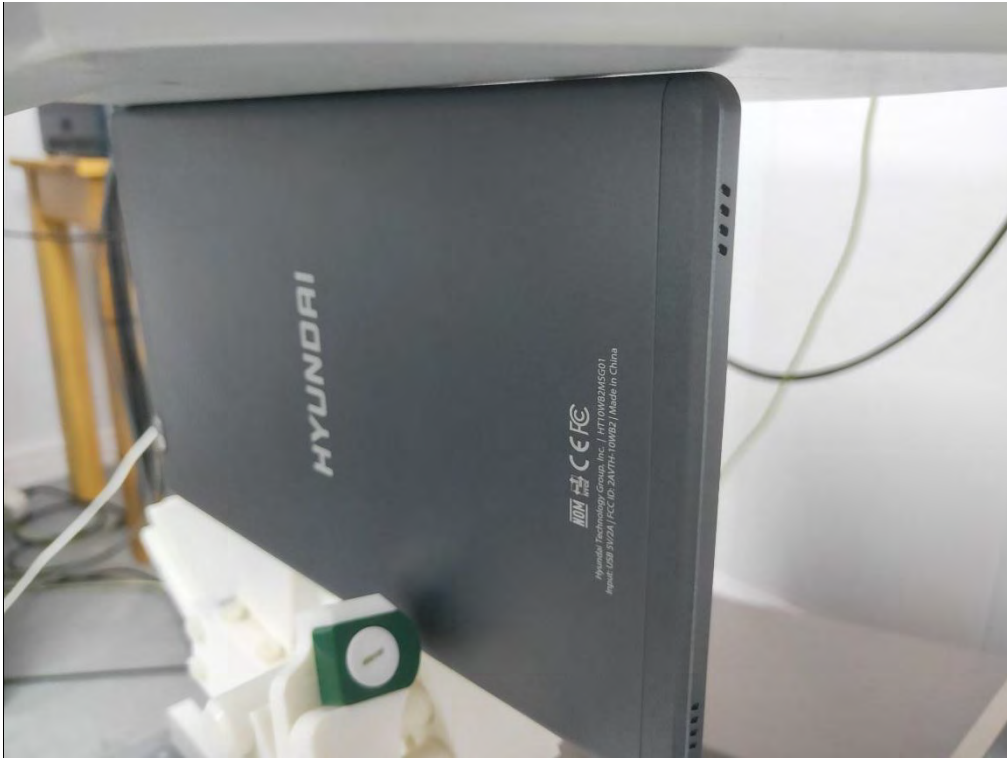
0mm body-worn Left Side Setup Photo
