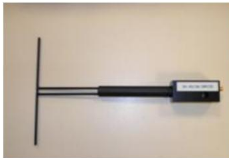
Figure 1 – Satimo COMOSAR Validation Dipole
