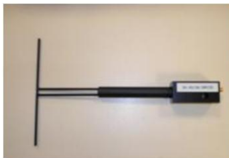
Figure 1 – Satimo COMOSAR Validation Dipole
