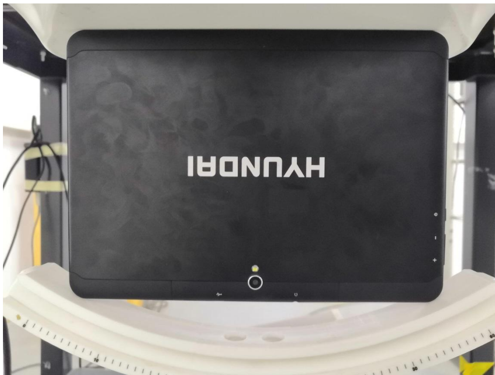
0mm body-worn Bottom Side Setup Photo (hotspot)
