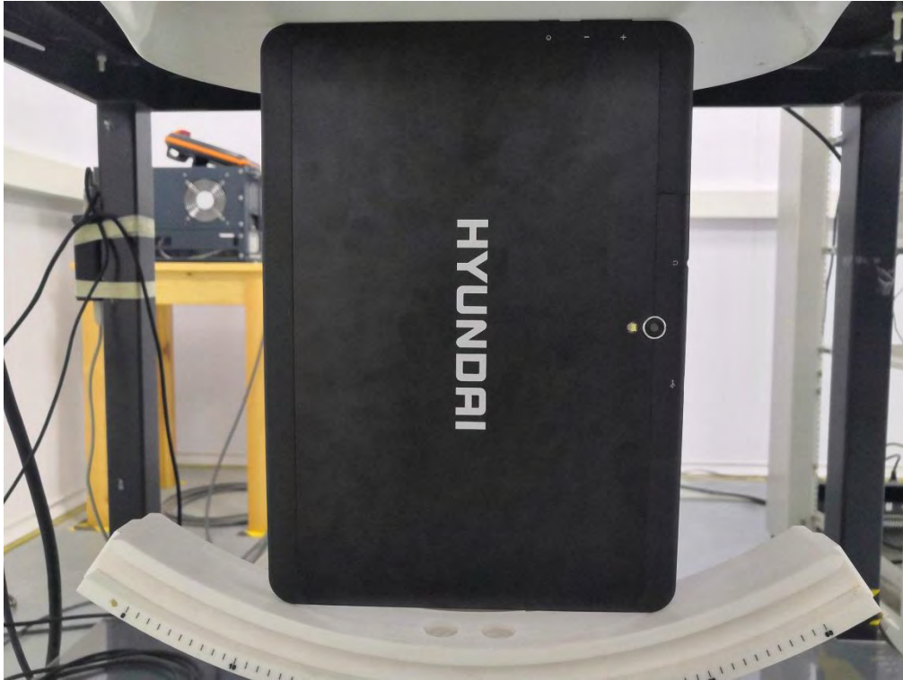
0mm body-worn Right Side Setup Photo (hotspot)
