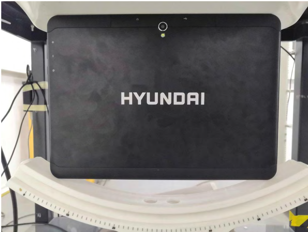
0mm body-worn Top Side Setup Photo (hotspot)
