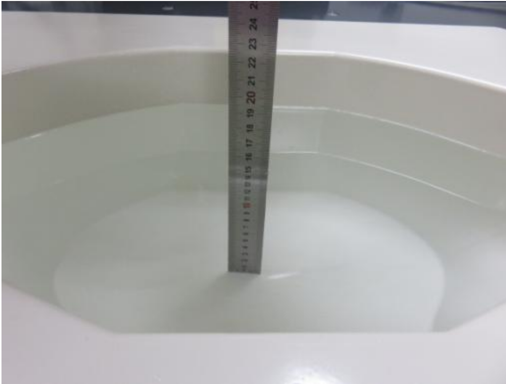
Photograph of the depth in the Body Phantom (750MHz, 16.1cm depth)
