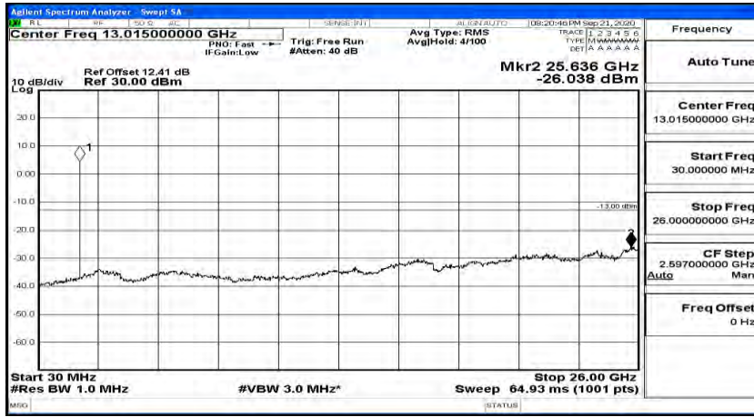
(Channel Bandwidth: 3 MHz)_LCH_16QAM_1RB#14
