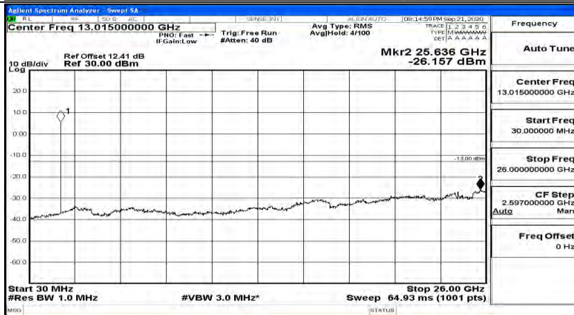
(Channel Bandwidth: 1.4 MHz)_LCH_QPSK_1RB#3
