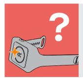
► If the wrist cannot be detected by the wrist sensor, the top of the Light-ring indicator will flash orange and the device will vibrate every few seconds.
