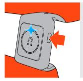
► Turn Romware ONE™ on by pushing the Multi-function button until the Light-ring indicator lights up blue. Let go of the button, the light ring indicator starts filling up blue while the device is starting.
