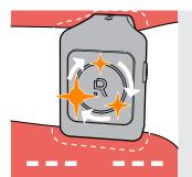
► When a worker response request is made, Romware ONE™ vibrates in an slow pattern of 3 buzzes. The light-ring indicator shows a slowly rotating orange light.
