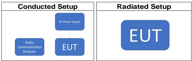
Note: Radio Communication Analyzer is placed in remote side for radiated test.
