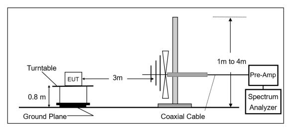
Radiated Emission Test Set-Up, Frequency Above 1GHz.
