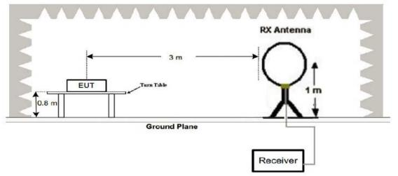
(2) Radiated Emission Test-Up Frequency 30MHz~1GHz
