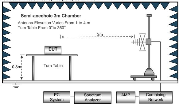
(C) Radiated Emission Test-Up Frequency Above 1GHz
