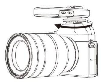
Tighten the hot shoe lock nut to secure the timelapse trigger
