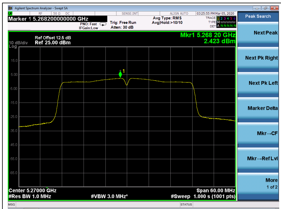
(Channel 54, 5270MHz, 802.11ac (VHT40))
