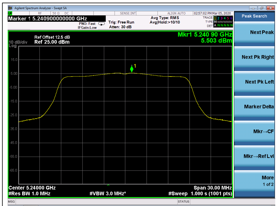
(Channel 48, 5240MHz, 802.11ac(VHT20))
