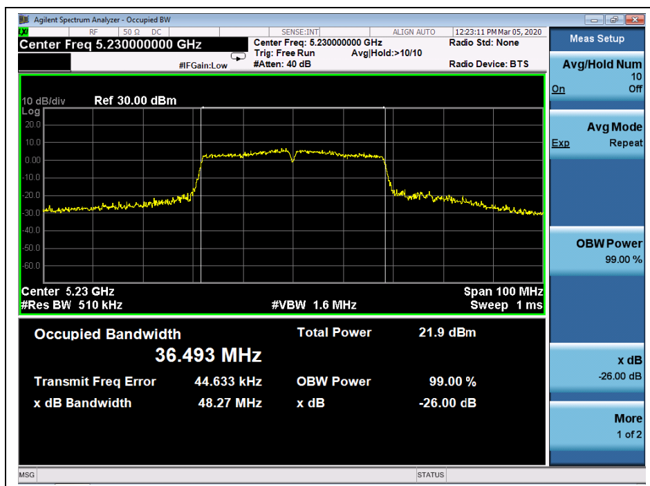
(Channel 46, 5230 MHz, 802.11ac(VHT40))
