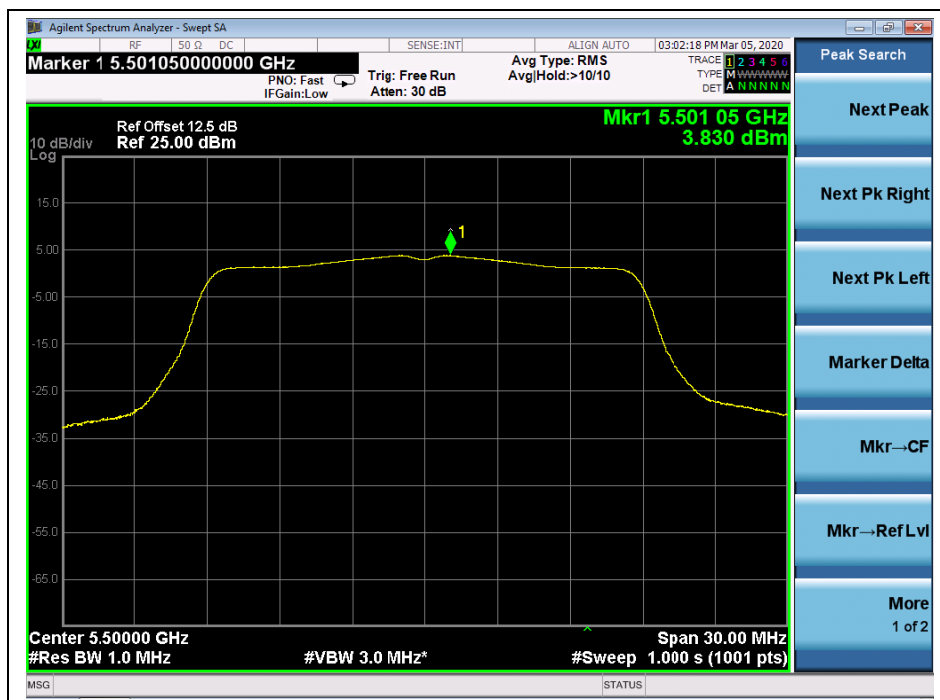
(Channel 100, 5500MHz, 802.11ac (VHT20))
