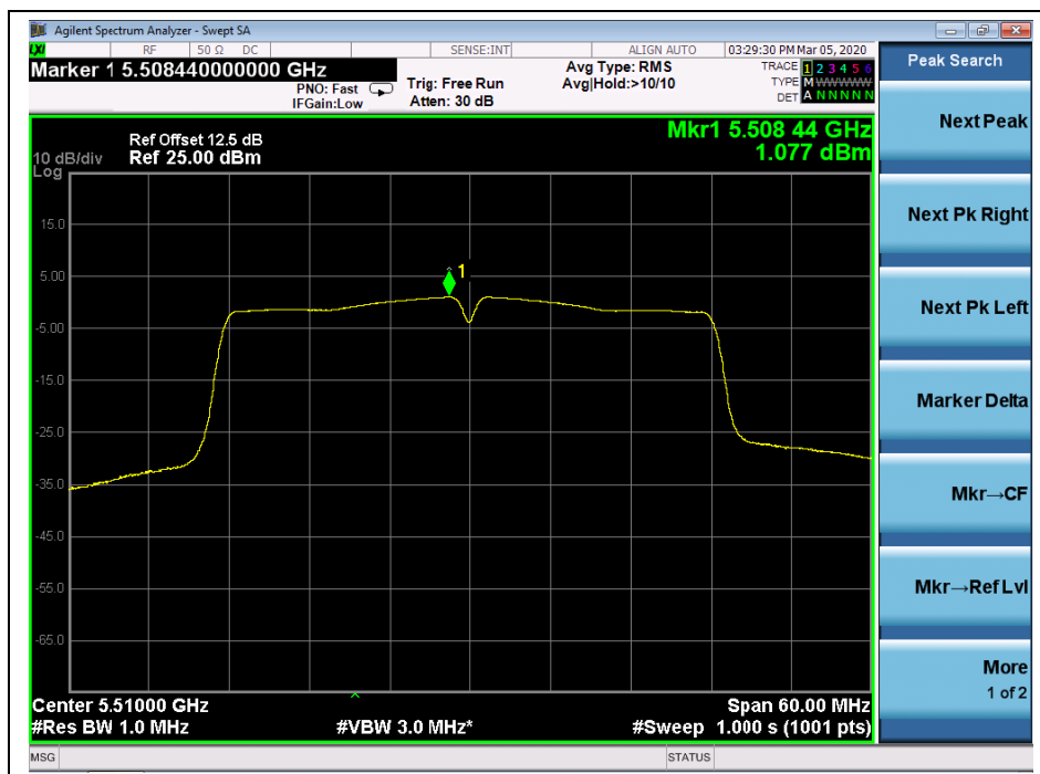
(Channel 102, 5510 MHz, 802.11ac (VHT40))
