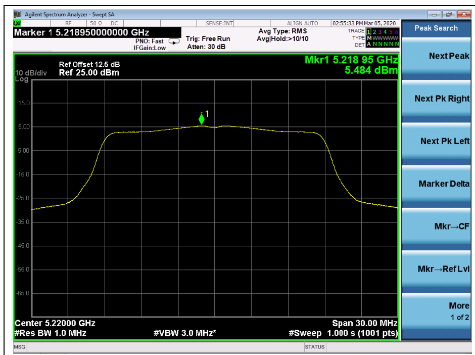
(Channel 44, 5220 MHz, 802.11ac (VHT20))
