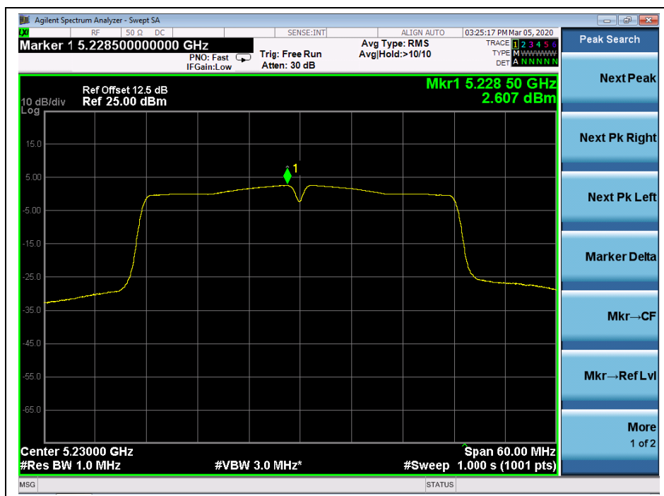
(Channel 46, 5230 MHz, 802.11ac (VHT40))
