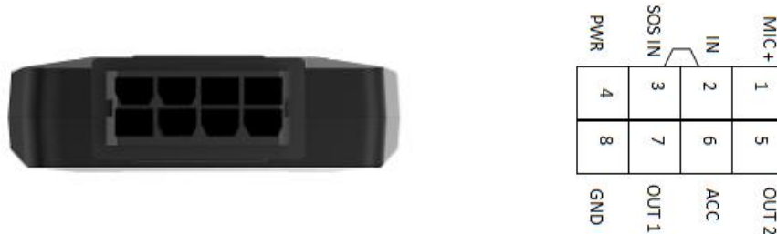
Figure 1. The 8 PIN connector on the QL-1000
