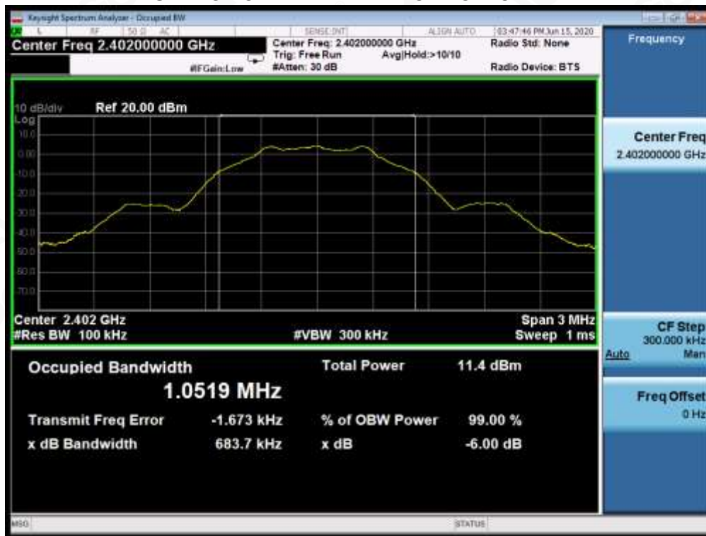
TEST PLOT OF BANDWIDTH FOR LOW CHANNEL
