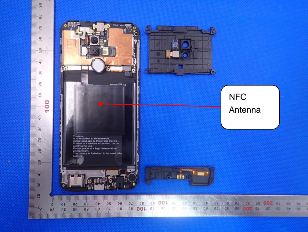
OPEN VIEW OF EUT(FIGURE 3)
