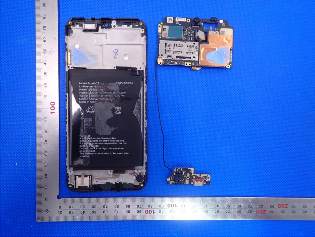
OPEN VIEW OF EUT(FIGURE 3)
