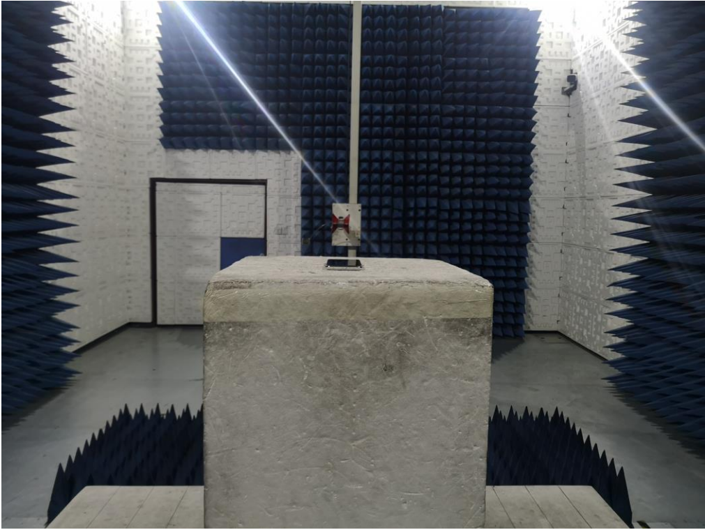
RADIATED EMISSION TEST SETUP ABOVE 1GHZ
