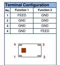
Function 1: Antenna fed from left Function 2: Antenna fed from right
