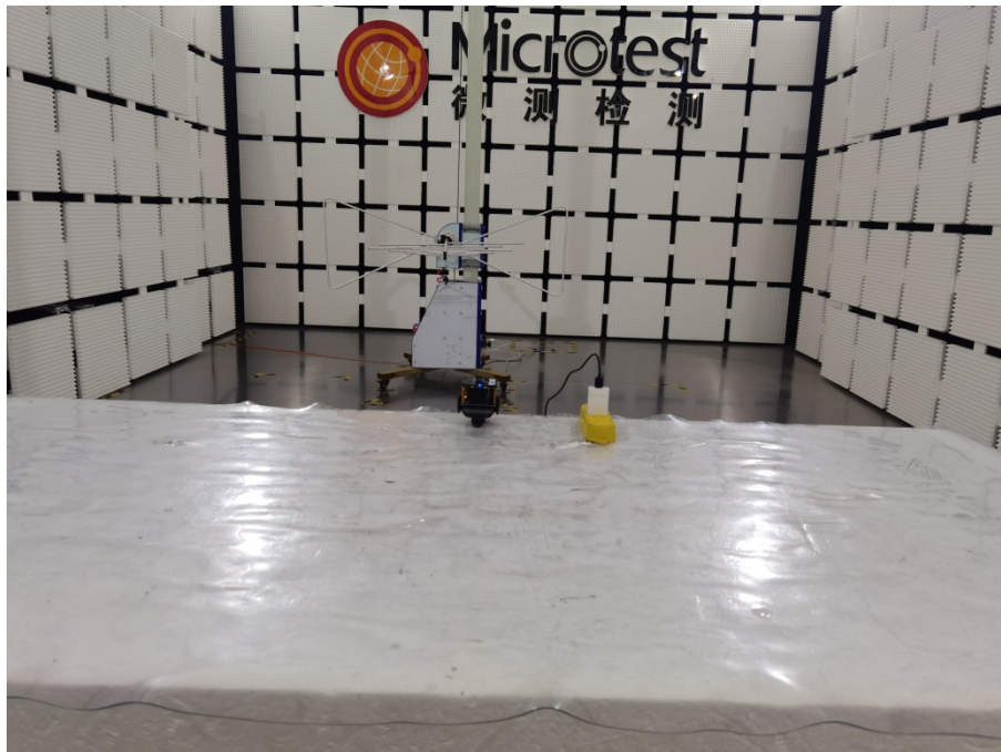
Radiated emissions – Blew 1 GHz
