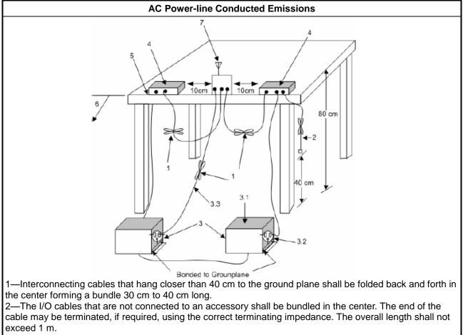
3—EUT connected to one LISN. Unused LISN measuring port connectors shall be terminated in 50  $\Omega$  loads. LISN may be placed on top of, or immediately beneath, reference ground plane.
