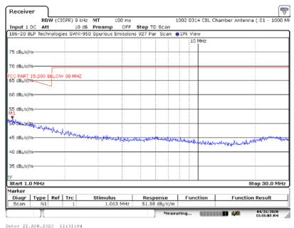
A1.1.3.2. Measurement Results: Perpendicular Receive Antenna
