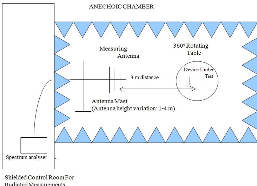
Radiated measurements setup from 1 GHz to 10 GHz:
