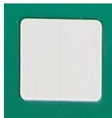
A white square has been included to include a QR code with the unique serial number included during mass production. The QR code would be laser engraved or stack using industrial grade stickers.
