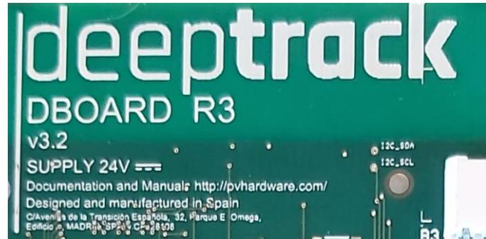
Commercial brand of manufacturer (DEEPTACK) is included, along as official address of the company. The name of the equipment (DBOARD R3) is also included along with input power supply. Additional information regarding documentation can be found in this part of the marking.
