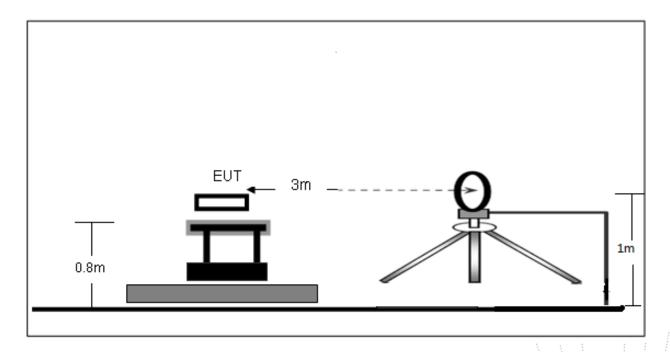
(B) Radiated Emission Test-Up Frequency 30MHz~1GHz
