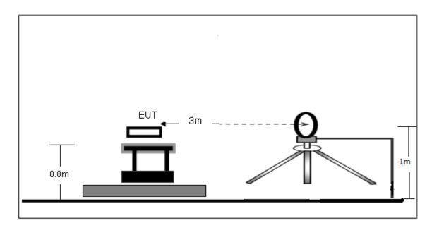
(B) Radiated Emission Test-Up Frequency 30MHz~1GHz
