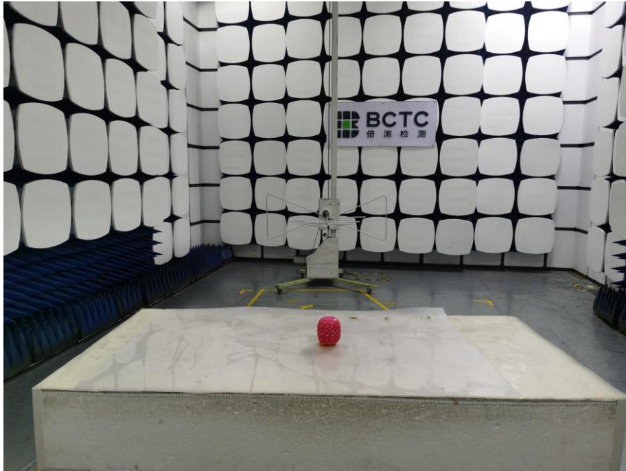
Radiated Measurement Photo (New IC+ Original Battery)
