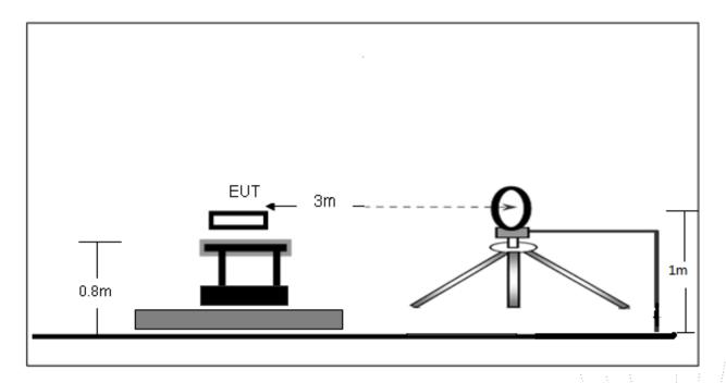
(B) Radiated Emission Test-Up Frequency 30MHz~1GHz
