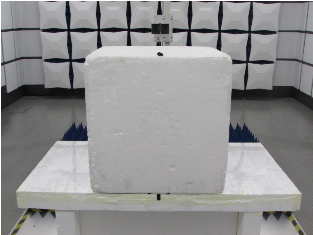
Radiated Emission Above 1GHz
