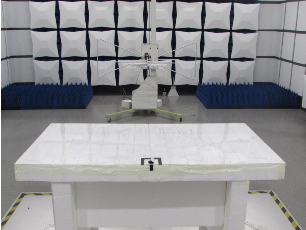
Radiated Emission Above 1GHz
