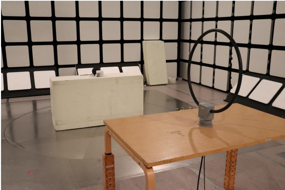
Photograph 6. Radiated Emissions 9kHz - 30 MHz
