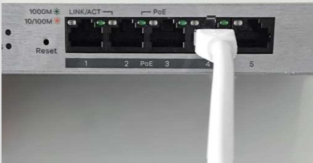
Figure 3: PoE Port of Switch, connected with Beacon
