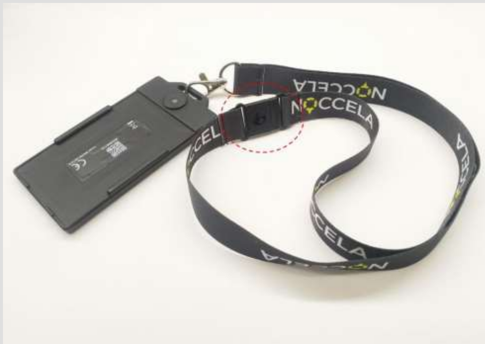
Figure 12: UWB Badge – lanyard with safety breaker feature
