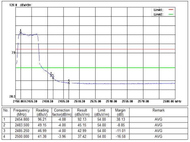
Mode:a; Polarization:Horizontal; Modulation:n; bandwidth:20MHz; Channel:High
