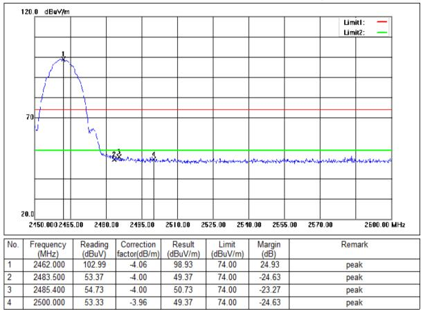
Mode:a; Polarization:Vertical; Modulation:b; bandwidth:20MHz; Channel:High
