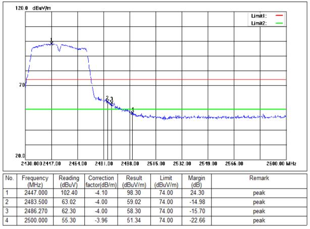
Mode:a; Polarization:Horizontal; Modulation:n; bandwidth:40MHz; Channel:High
