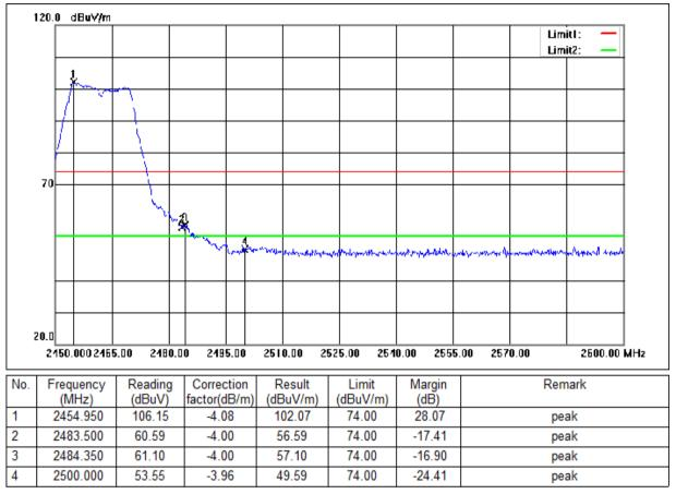
Mode:a; Polarization:Horizontal; Modulation:g; bandwidth:20MHz; Channel:High
