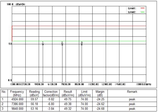
Mode:a; Polarization:Vertical; Modulation:b; bandwidth:20MHz; Channel:High
