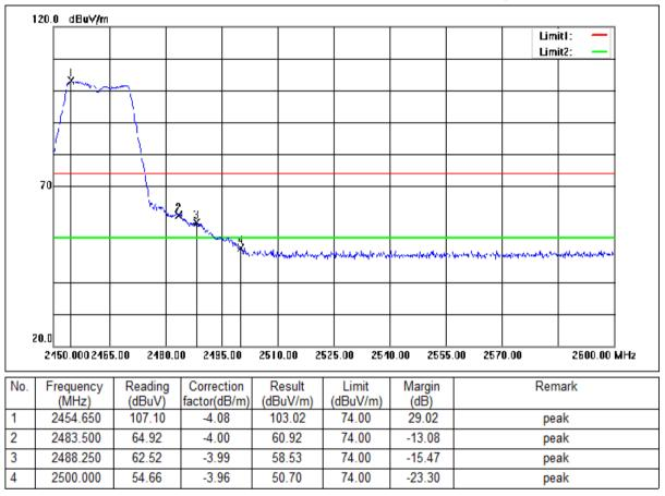
Mode:a; Polarization:Vertical; Modulation:n; bandwidth:20MHz; Channel:High
