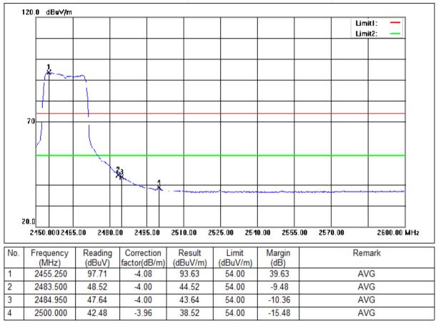
Mode:a; Polarization:Vertical; Modulation:g; bandwidth:20MHz; Channel:High
