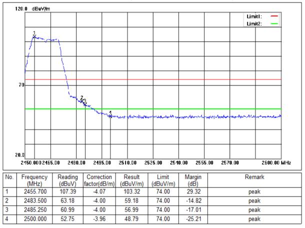
Mode:a; Polarization:Vertical; Modulation:g; bandwidth:20MHz; Channel:High
