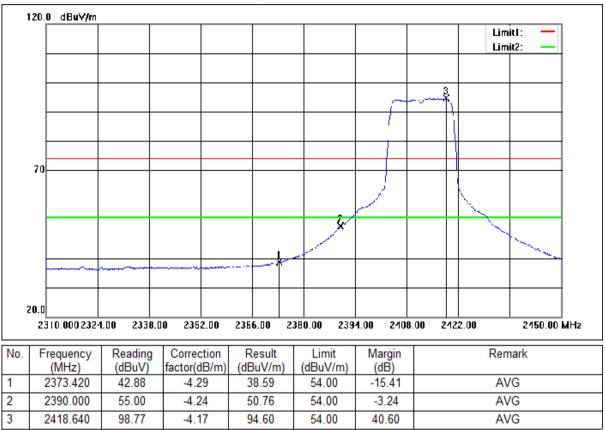
Mode:a; Polarization:Vertical; Modulation:g; bandwidth:20MHz; Channel:Low
