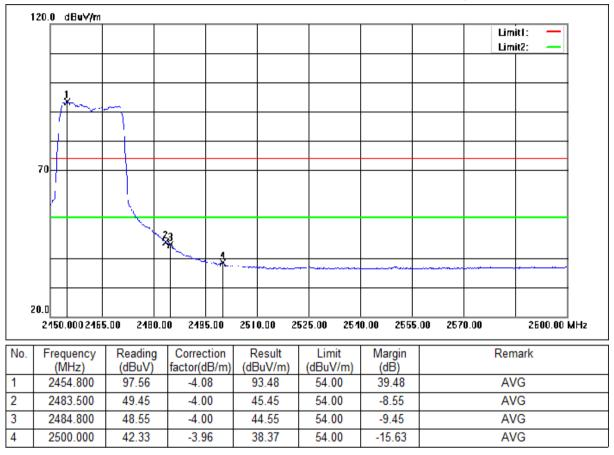
Mode:a; Polarization:Vertical; Modulation:n; bandwidth:20MHz; Channel:High
