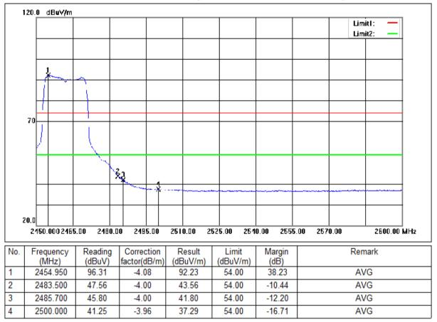
Mode:a; Polarization:Horizontal; Modulation:g; bandwidth:20MHz; Channel:High
