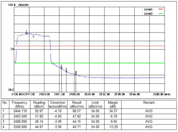
Mode:a; Polarization:Horizontal; Modulation:n; bandwidth:40MHz; Channel:High
