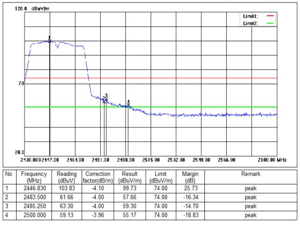
Mode:a; Polarization:Vertical; Modulation:n; bandwidth:40MHz; Channel:High
