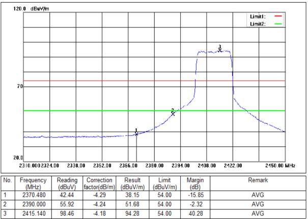
Mode:a; Polarization:Vertical; Modulation:n; bandwidth:20MHz; Channel:Low
