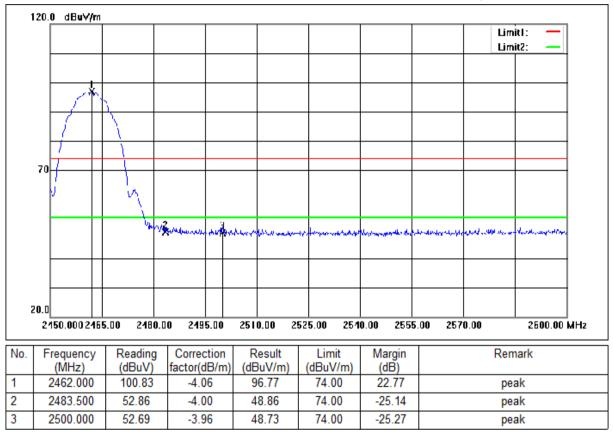
Mode:a; Polarization:Horizontal; Modulation:b; bandwidth:20MHz; Channel:High
