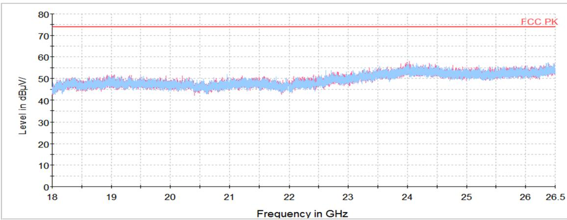
**Simultaneously\_BT,GFSK(2 480 MHz)+ BLE,GFSK(2 402 MHz)**
