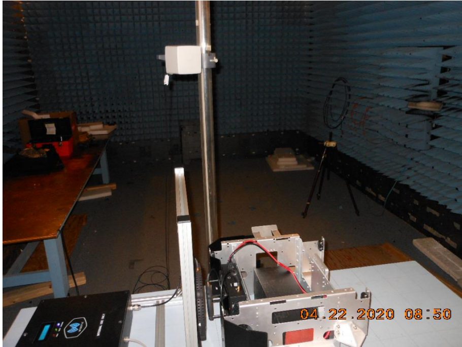
Example Position for Spatial Average – “20cm max + 80” position shown
