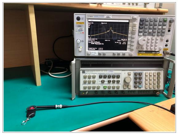
Radiated Electric Field Emissions Test (Below 1 GHz)
