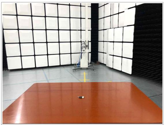
Radiated Electric Field Emissions Test (Above 1GHz)
