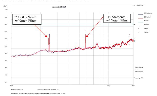
S.A. Correction Corrected Antenna Antenna Turntable **Frequency** Limit Margin Reading **Factor** Amplitude Height **Polarity Azimuth** Comment (MHz)  $(dB\mu V/m)$ (dB) (dBuV) (dB/m) (dBµV/m) (cm) (H/V)(degrees) 16576.52 41.22 25.08 66.3 219 V 238 -17.7 Peak 84 16576.52 30.84 25.08 55.92 204 Η 28 64 -8.08 Average
