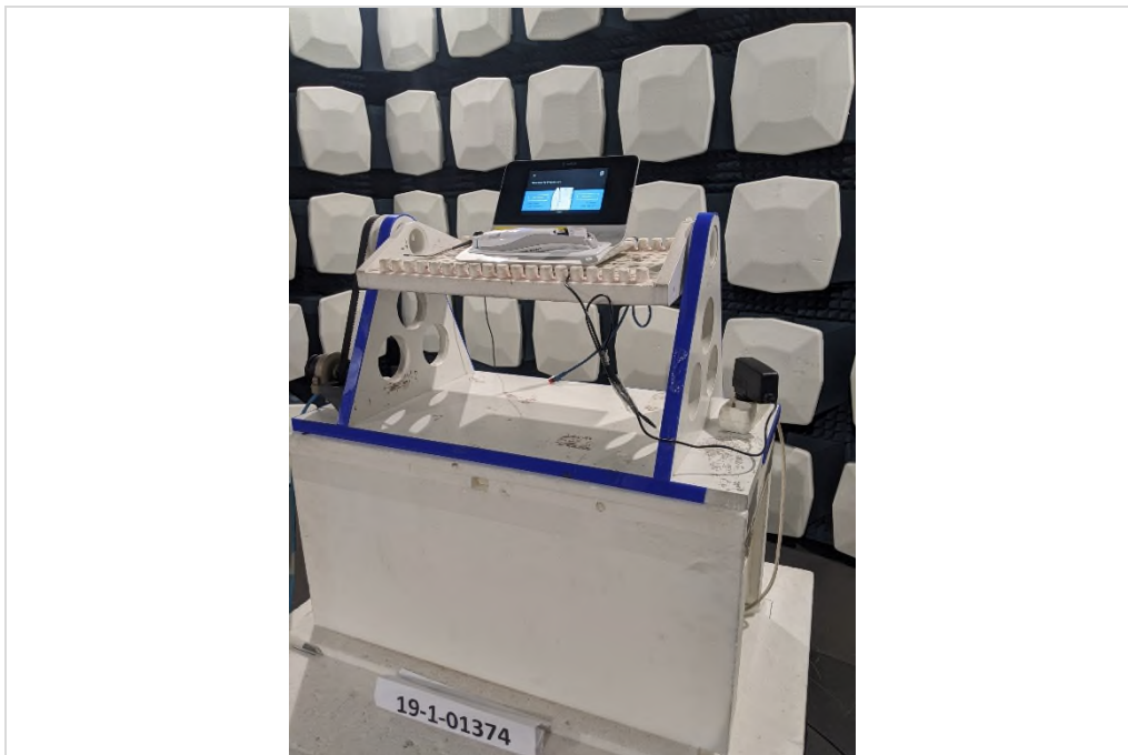
Photograph 8: EUT Test Setup in the anechoic chamber, Radiated interference field strength, close-up view
