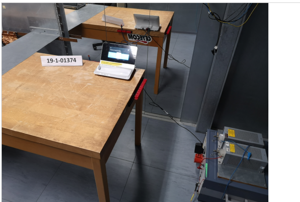
Photograph 6: EUT Setup Conducted emissions on AC-Power lines
