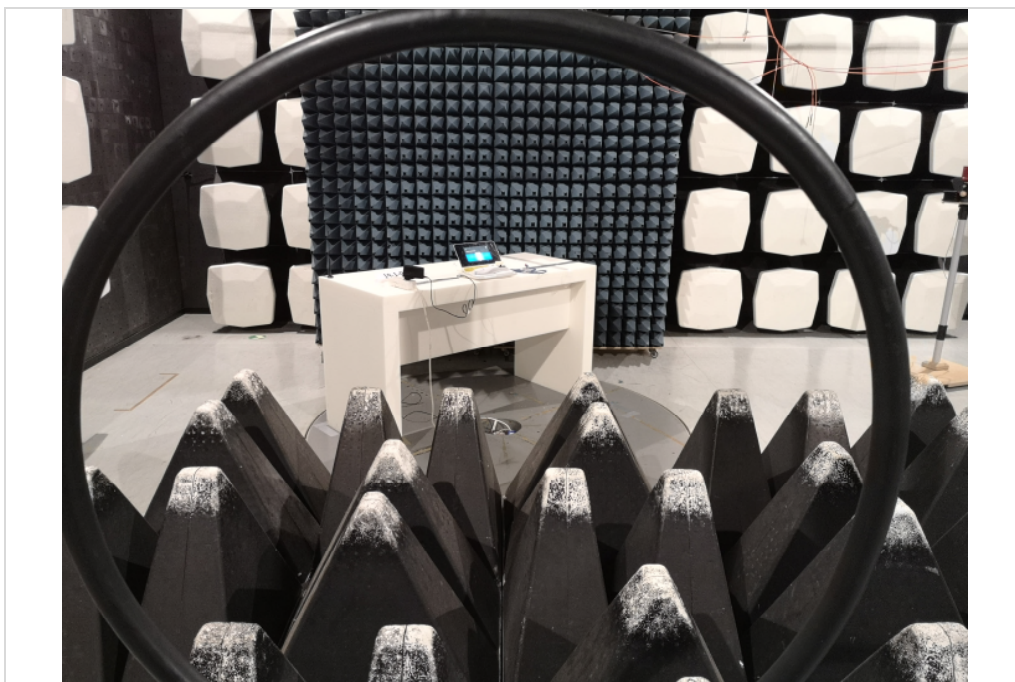
Photograph 9: EUT Setup Magnetic Field Measurements in the Semi anechoic chamber Long shot view
