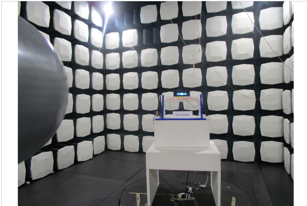
Photograph 1: EUT Test Setup in the anechoic chamber, Radiated interference field strength, long shot view
