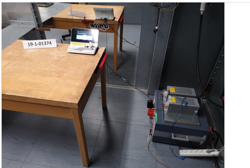
Photograph 12: EUT Setup Conducted emissions on AC-Power lines
