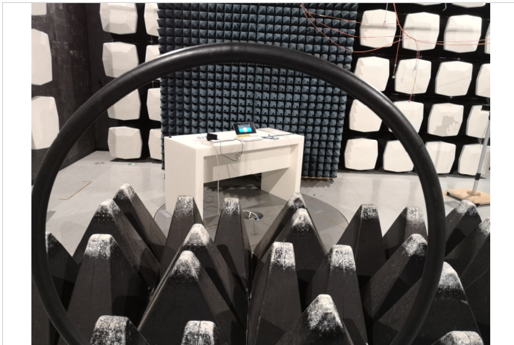
Photograph 3: EUT Setup Magnetic Field Measurements in the Semi anechoic chamber, Long shot view
