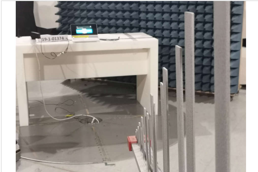
Photograph 5: EUT Test Setup in the semi-anechoic chamber, Radiated interference field strength
