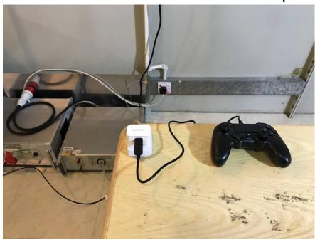
Radiated Emissions (30MHz-1GHz) Test Setup
