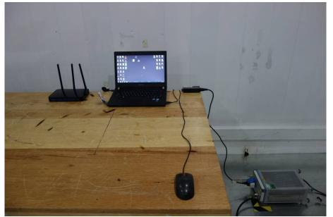
1.1 Conducted Emissions at AC Power Line (150kHz-30MHz) Test Setup
