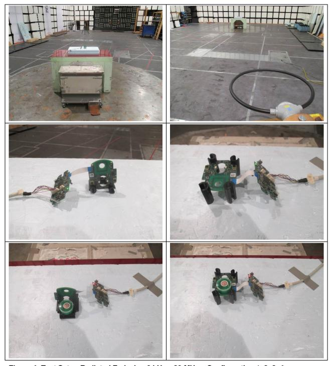
Figure 4: Test Setup Radiated Emission 9 kHz - 30 MHz - Configuration 1, 2, 3, 4
