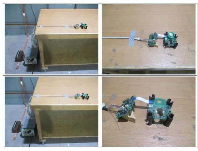
Figure 1: Test Setup Conducted Emissions (150 kHz - 30 MHz) - Configurations 3, 4, 5
