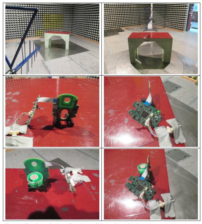
Figure 3: Test Setup Radiated Emission 30 MHz – 1 GHz – Configurations 1, 2
