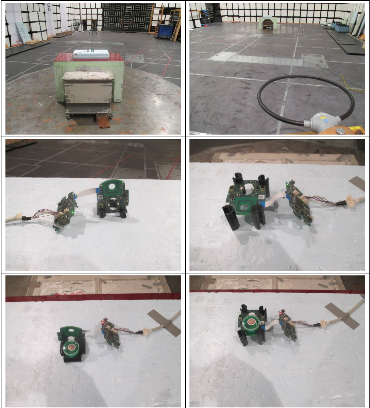
Figure 7-24: Test Setup Radiated Emission 9 kHz – 30 MHz – Configuration 1, 2, 3, 4
