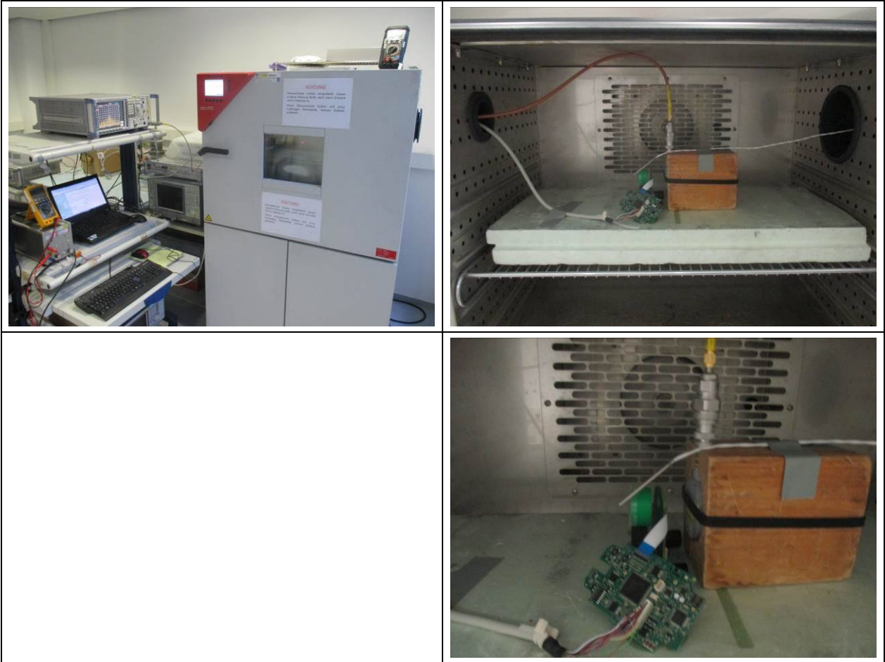
Figure 7-25: Test Setup – Frequency Stability with voltage or/and Temperature variation – Configuration 2
