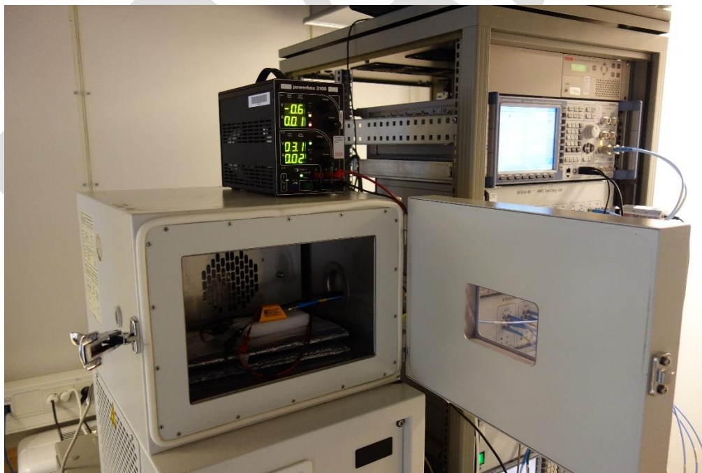
Picture 1: EUT placement– CTE system
