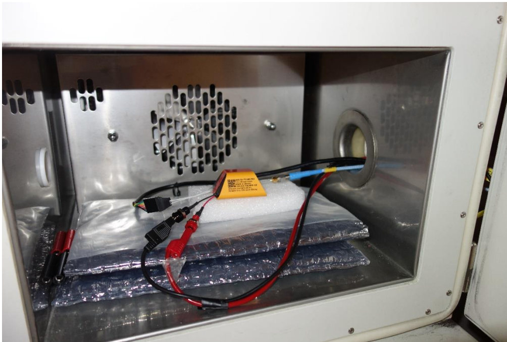
Picture 1: EUT placement inside temperature chamber – CTE system
