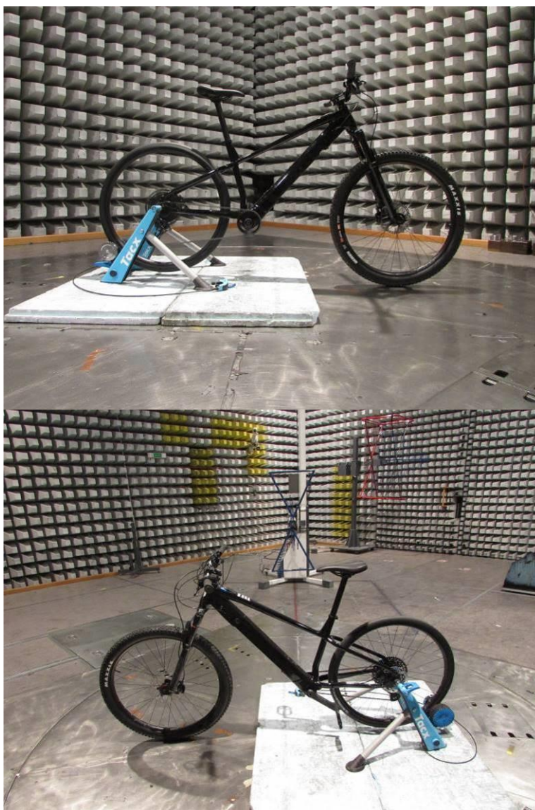
Figure 6-2: test setup for Radiated disturbances 30 MHz to 1000 MHz
