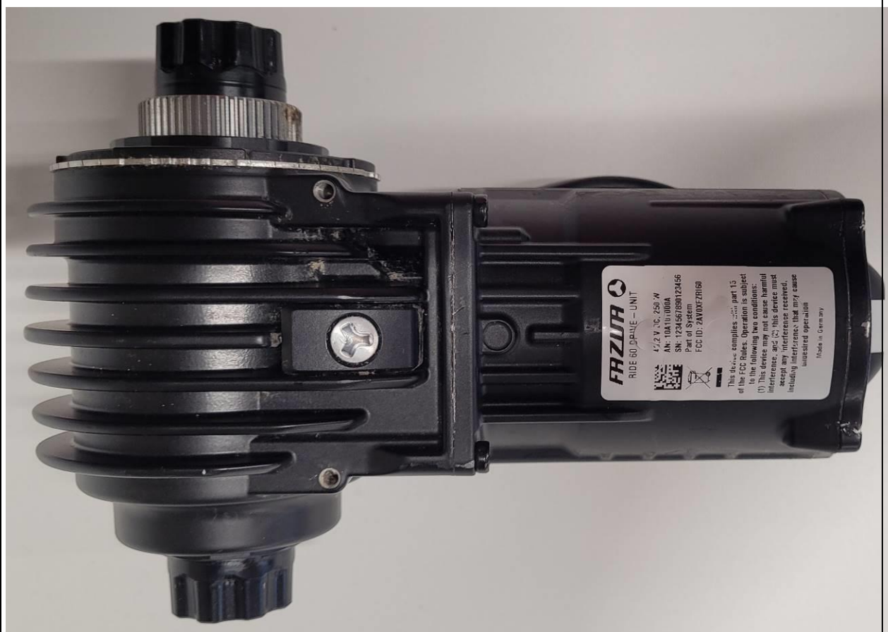
Figure 4-5: Motor: DRIVE UNIT, with type product label FCC information
