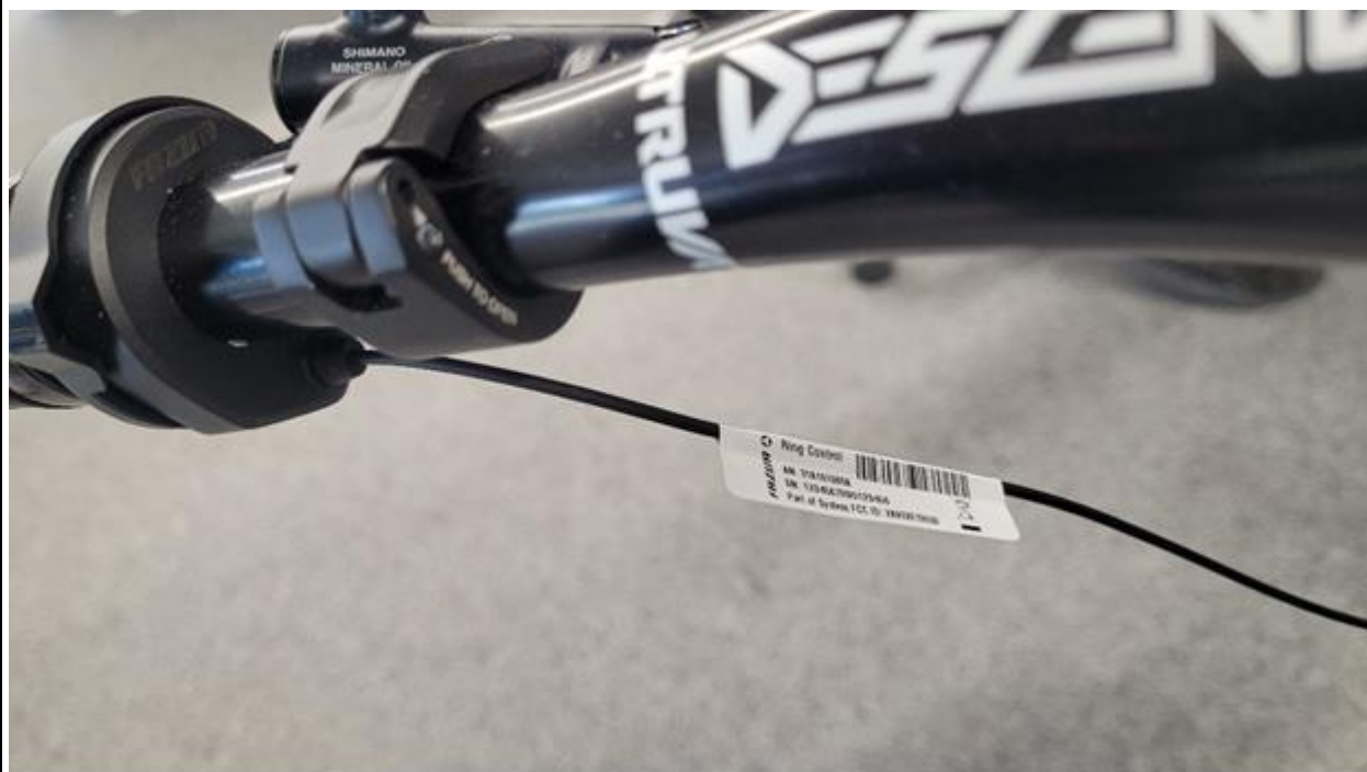
Figure 4-10: Remote: RING CONTROL, with product label incl. FCC information
