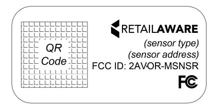
The label will be located on the long edge of the device, transducer side. Note that the FCC part 15 statement does not fit anywhere on the device without reducing the font size below the required 4pt font minimum. The bottom of the enclosure is removable and not an option for labeling.
