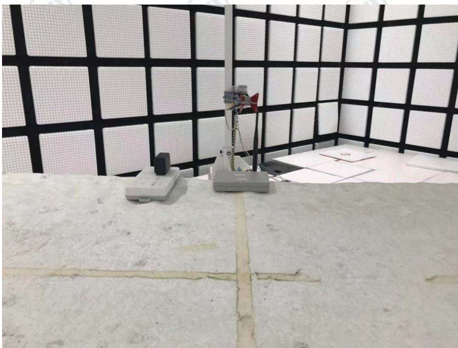
Radiated spurious emission Test Setup-2(Above 1GHz)
