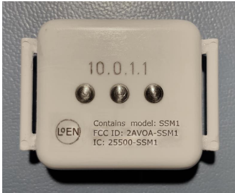
Bottom View of PLI Bracelet, Showing Laser Etched FCC and IC Markings
