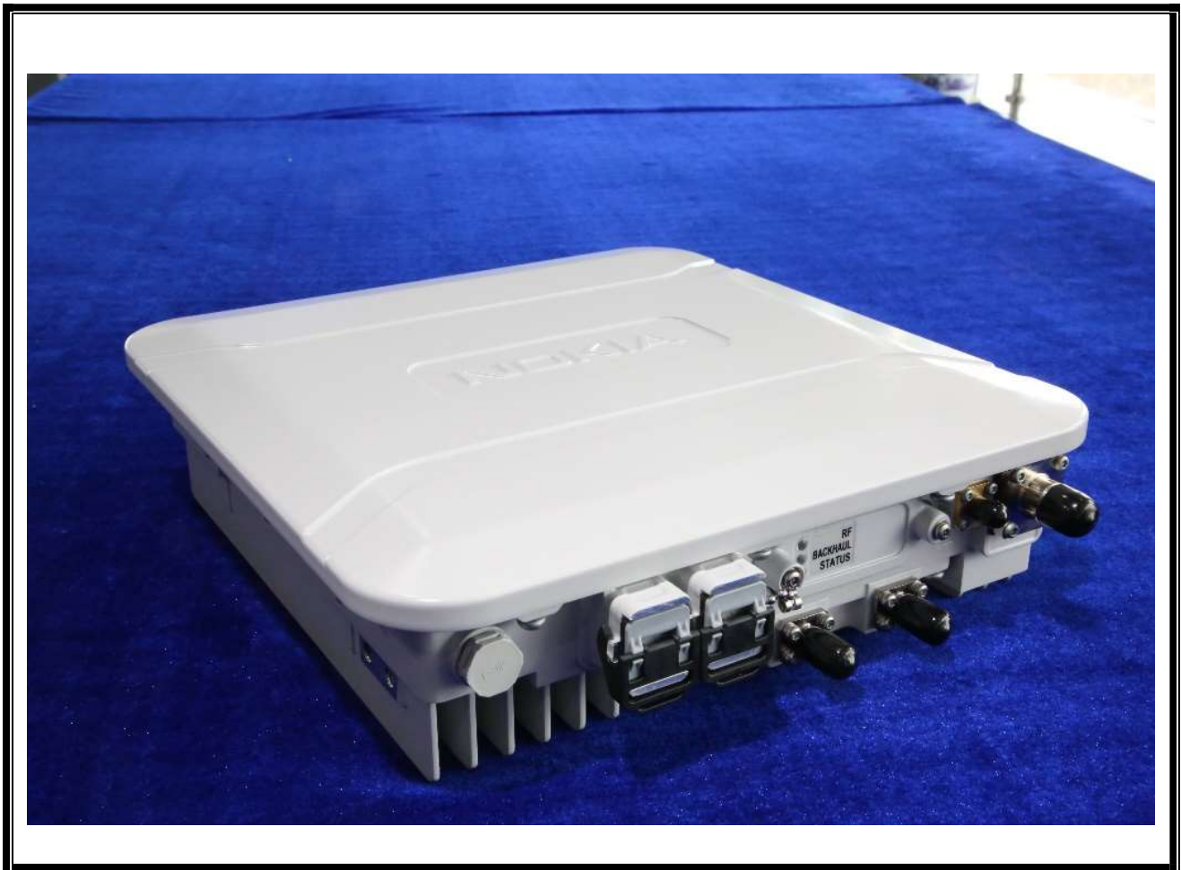
Allover photo Outline dimension : 273.5mm (L)X 269.4mm(W) X 74.3mm(H)
