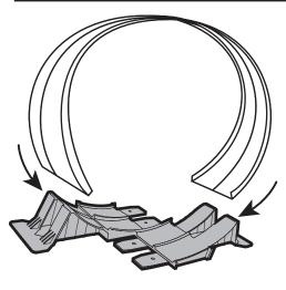
The loop track is the 27 inch piece of track without holes cut into the end.
