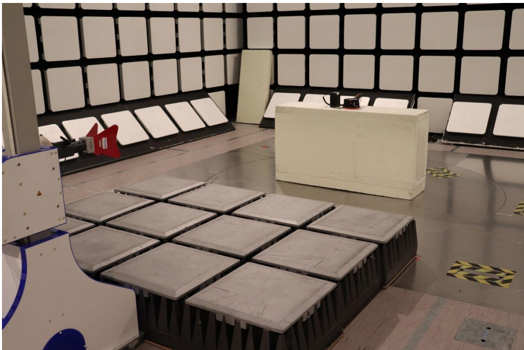
Photograph 8. Radiated Emissions 1 – 18 GHz
