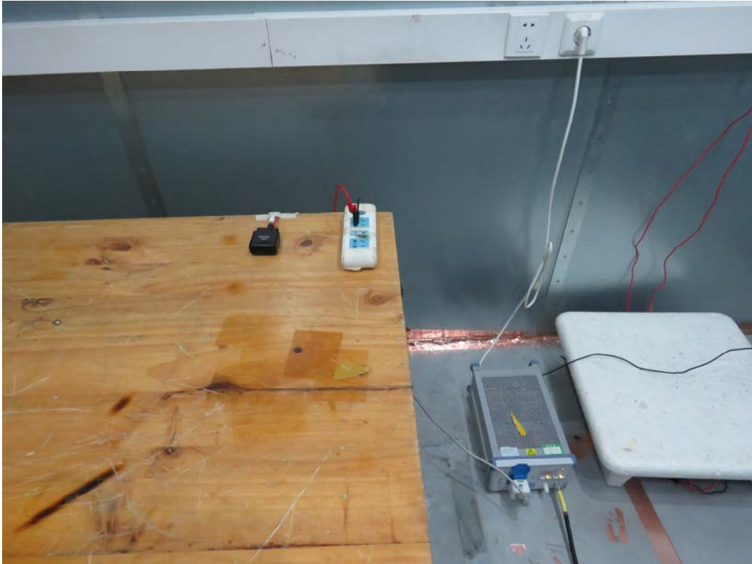
Picture 2 Conducted Emission Test Setup
