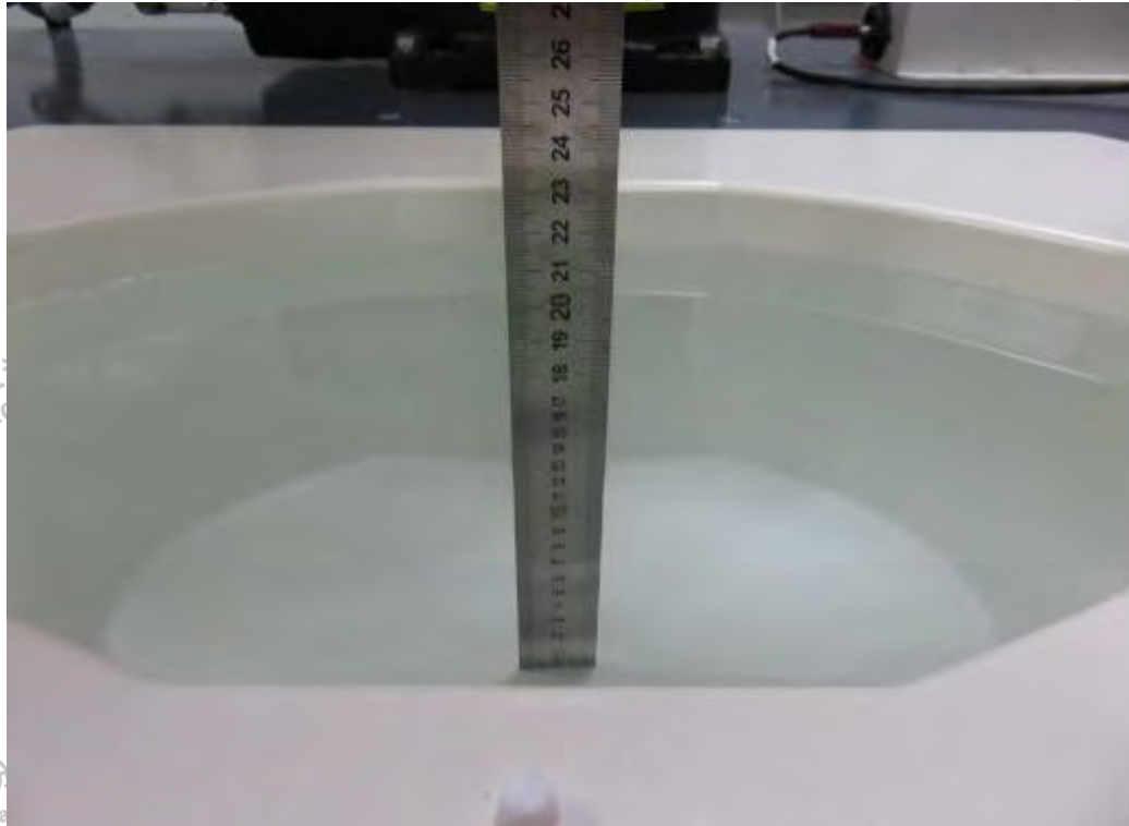
Photograph of the depth in the Body Phantom (2450MHz, 15.8cm depth)
