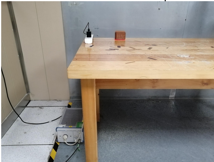
Conducted Emissions Test Setup
